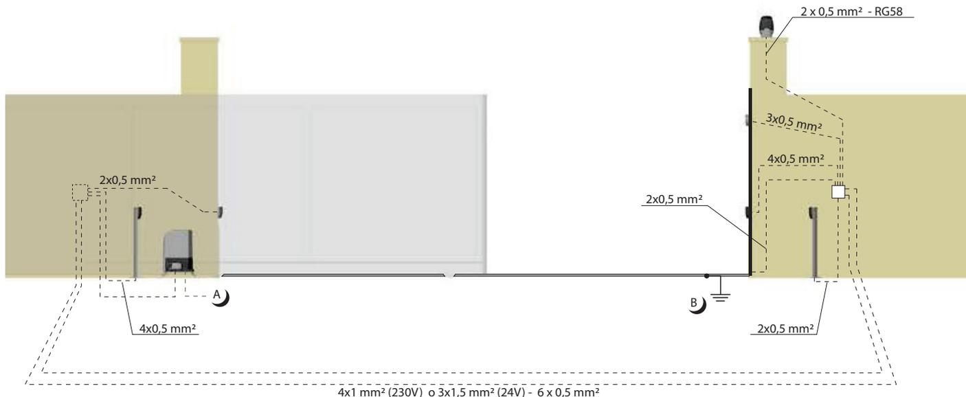
EXAMPLE OF A TYPICAL INSTALLATION
